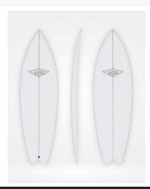
With the Soul Budha model, we aimed to create a livelier feel than a retro fish by incorporating aspects of a high-performance modern surfboard. We took the "Retro" fish, thinned out the rails, which gave us grip for harder and faster turns, changed the rocker for a more modern performance feel, while maintaining the flat deck for paddling advantages.
